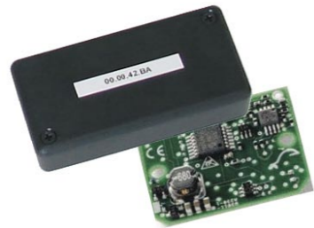
Fig. Radio sensor with self-sufficient power supply
